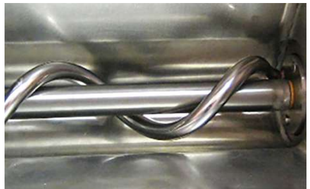
Spiral in stainless steel inside the tank.
