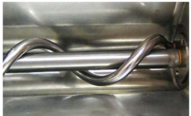
Spiral in stainless steel inside the tank.
